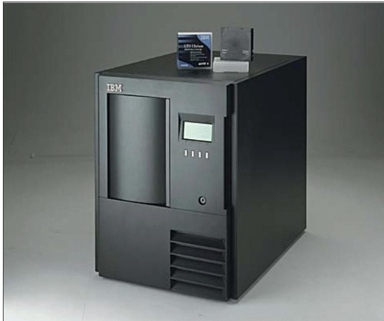
*Figure 4-5 IBM TotalStorage Ultrium Scalable Tape Library 3583*
